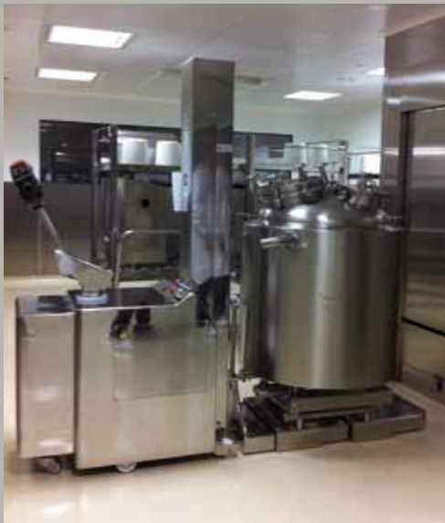
Alimentation autoclave Autoclave loading system
